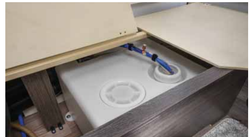
Fresh water tank with lockable tank cap and integrated overflow/emptying nozzle
