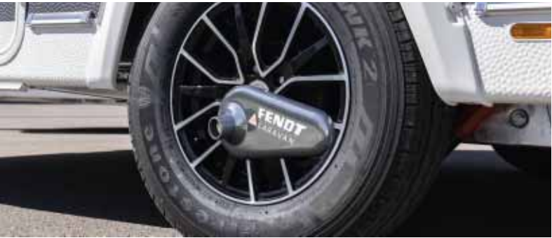
Fullstop mechanical anti-theft protection *
