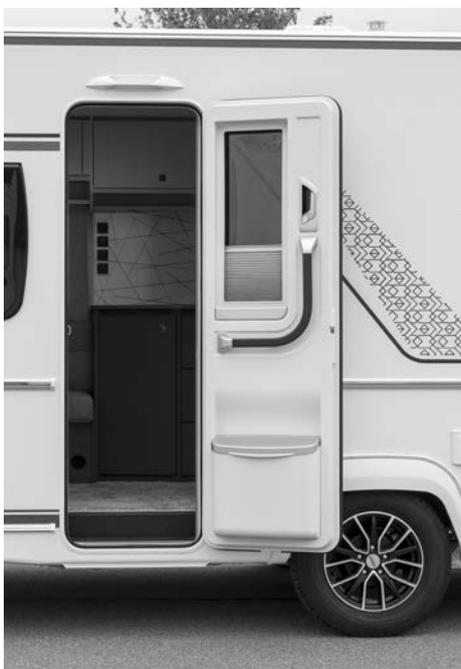
The external entry door has been designed for use in leisure vehicles. There are two different versions:
