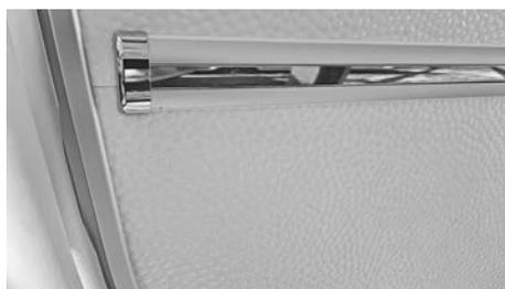
To insert the tent keder at the front or rear end, the guide rail for the outer tent has been milled out at the edge of the ornamental strip.
