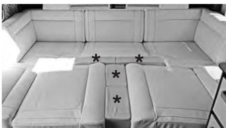
**Converting a round seating arrangement into a bed (Diamant)**
