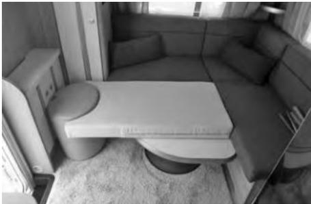
**Converting the L-shaped seating arrangement into a bed (optional extra for Bianco 465 SGE)**
