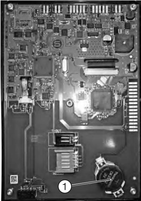
Circuit board (reverse side) of TFT display
