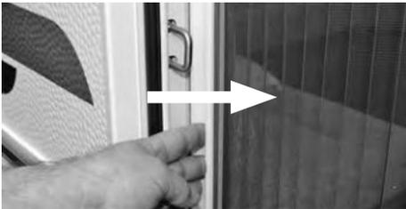
Always hold the rail in the middle to operate the insect screen door and pull it back across the entire width of the door opening until it can longer be moved.
