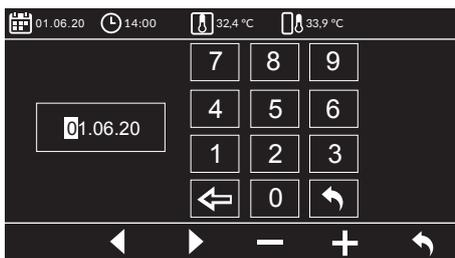
Press lightly on the Time display next to the Alarm Clock icon to navigate to the Setting menu for the timer.
