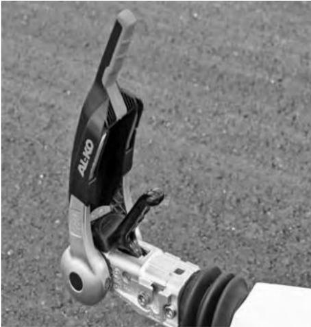
The caravan is equipped with an anti-rolling coupling in accordance with ISO 11555-1. This safety coupling stabilises the caravan while driving and ensures better driving performance.
